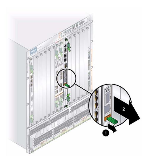
8. Replace the AMC with another AMC (FIGURE 1-7) or install a filler panel.
